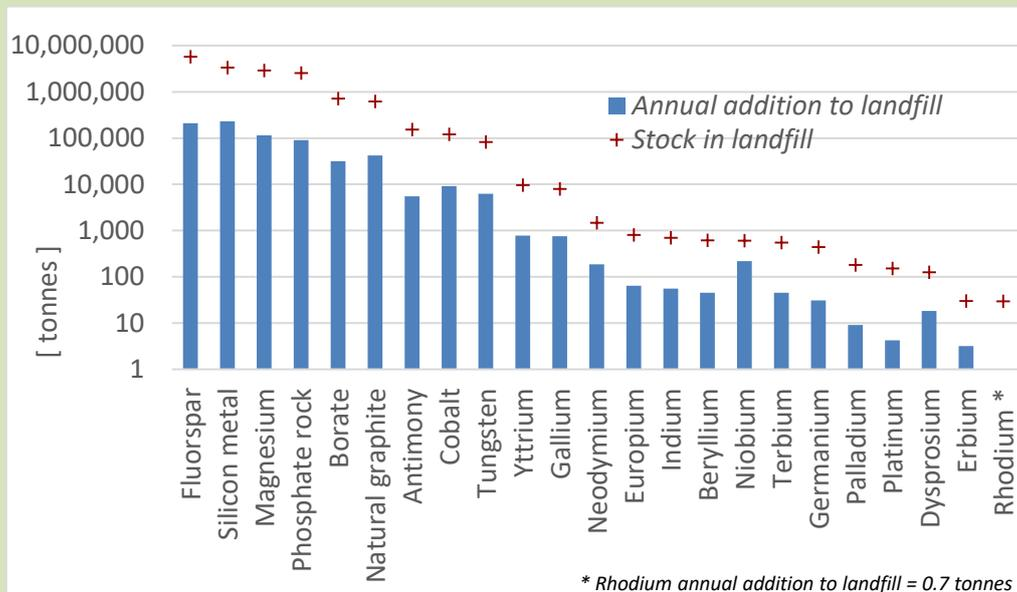
**Figure 11.** Estimated amounts of various CRMs as 'Annual addition to stock in landfills in the EU' and 'Stock in landfill in the EU'. *Source:* JRC elaboration based on 2015 MSA study<sup>78</sup>.
