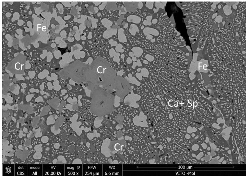
**Figure 22:** Morphological aspects of carbon steel EAF slags. Fe = Fe-oxides, Cr = Cr-rich spinel minerals, Ca = Ca-silicates, Sp = Cr-poor spinel minerals
