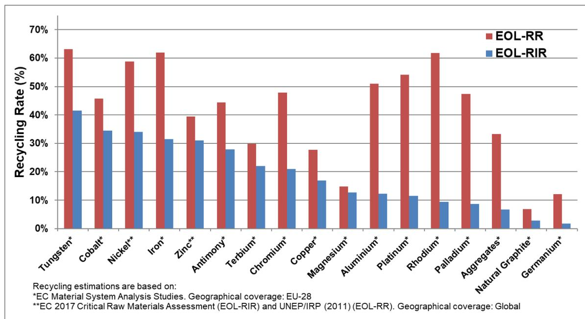
**Figure 3.** Current contribution of recycling to meet EU demand for CRMs: end-of-life recycling Input Rate (EOL-RIR). Source: JRC elaboration based on Deloitte Sustainability (2015 and 2017)<sup>21,22</sup>.
