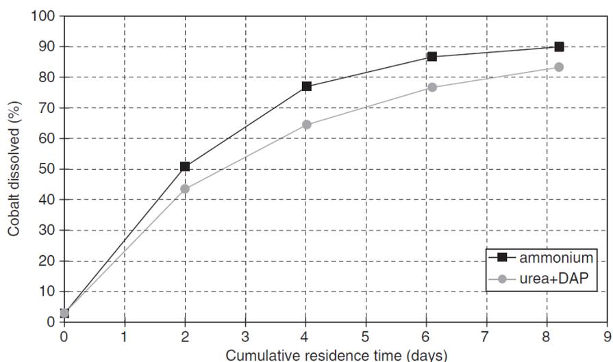
**Figure 26:** Bioleaching kinetics - Influence of the nitrogen source on the kinetics of cobalt dissolution in continuous laboratory scale bioleaching unit (100 L) (d'Hugues et al, 1997)
